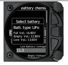
Alternatively you can manually change the Full Voltage, Low Battery Voltage and Empty Voltage if your battery type is not listed.
