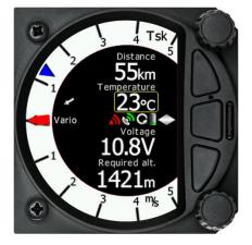
The navigation boxes in this second task page can be changed using the quick access menu and selecting **NavBox**. You can make changes to the NavBoxes as described in chapter.
