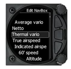
Select the required NavBox and then save this with a short press of the bottom rotary knob. Repeat the process for any other NavBox that needs to be changed.
