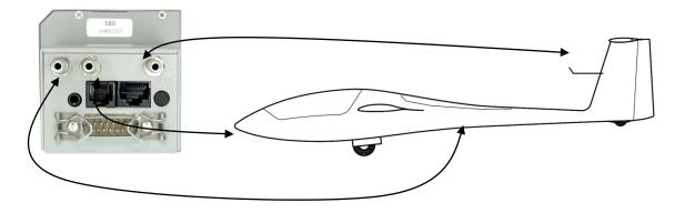
If the P<sub>total</sub> and Static are connected the wrong way around there will be no integrator (average climb) and speed to fly indication during the flight.
