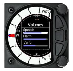
The lower rotary knob is used to adjust settings, within the current screen display or within menus. With the lower rotary pushbutton is possible to toggle between MC, Ballast and Bugs settings. In all other menus, this knob is used for setting values and editing texts.
