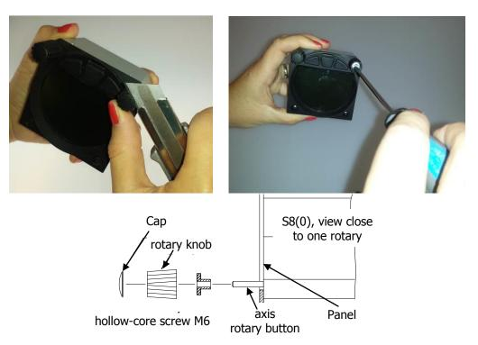
Remove the two rotary knob caps with a knife or flat screw driver, then hold each knob and unscrew it.
