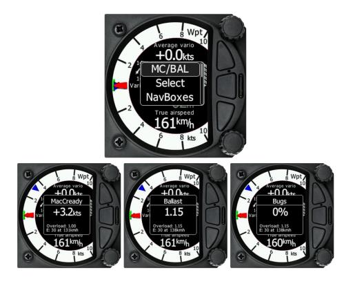
Rotate the bottom knob to modify any setting. Next, check the safety altitude (height above destination, arrival altitude) setting.
