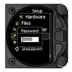
Turn the bottom rotary Knob to set the character and then press the enter key (bottom key) to move to the next character to the right. Press the escape key to move back to the left. When you have finished editing, press the Enter key. Short-press on the bottom rotary knob to enter or exit an edited field ("control").
