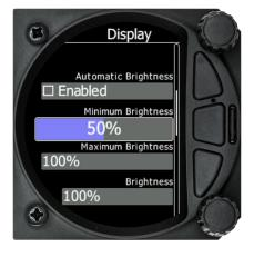
With a push of the lower rotary button you can activate the slide control and then with rotation of the knob you can select the preferred value and confirm it with the push button.
