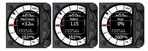
To change the MacCready value, rotate the bottom rotary knob and press on MC/BAL. A short press on the bottom rotary knob moves from MacCready to the Ballast box and pressing the bottom rotary knob again will open the Bugs box. If no action is performed for 3 seconds, the box will close.
