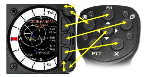
Remote stick is also connected to CAN bus. On S8(0)/S10(0) is provided special menu to register remote stick. Device must be registered in case of double seat device, there is possible to have two remote stick, one registered on front and another on rear device.
